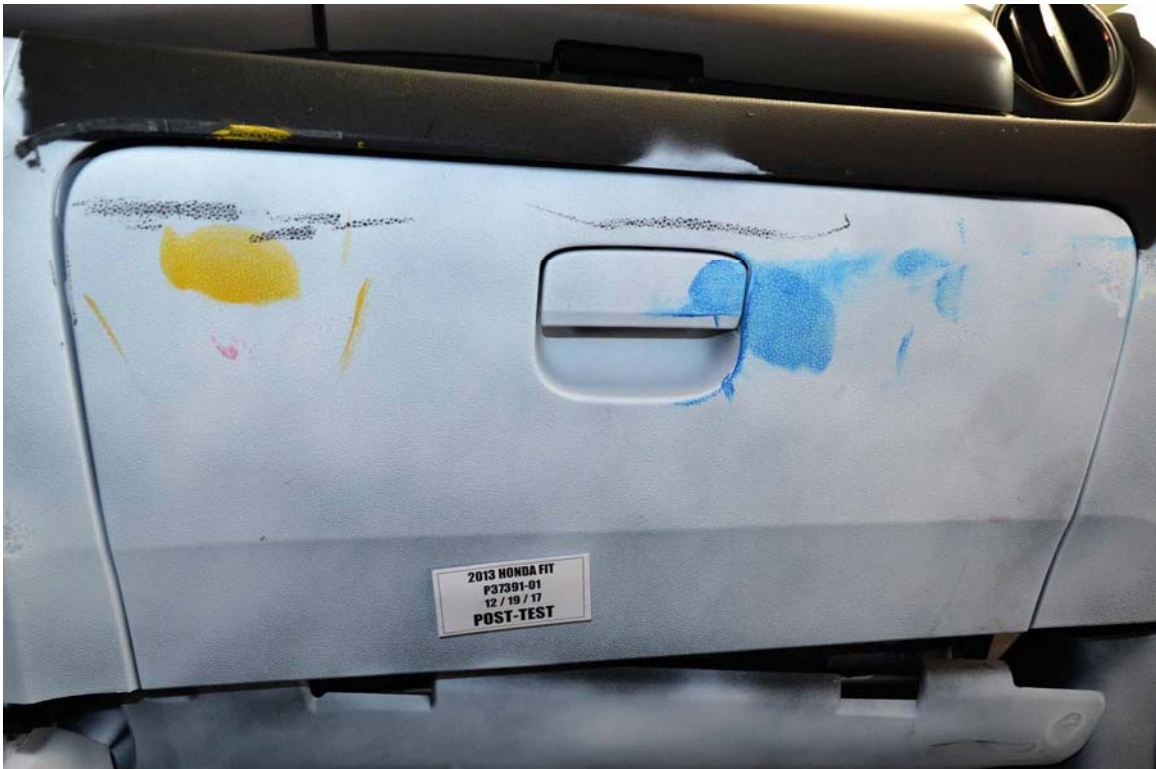
FIGURE 54. Post-Test Passenger Dummy Contact with Knee Bolster
