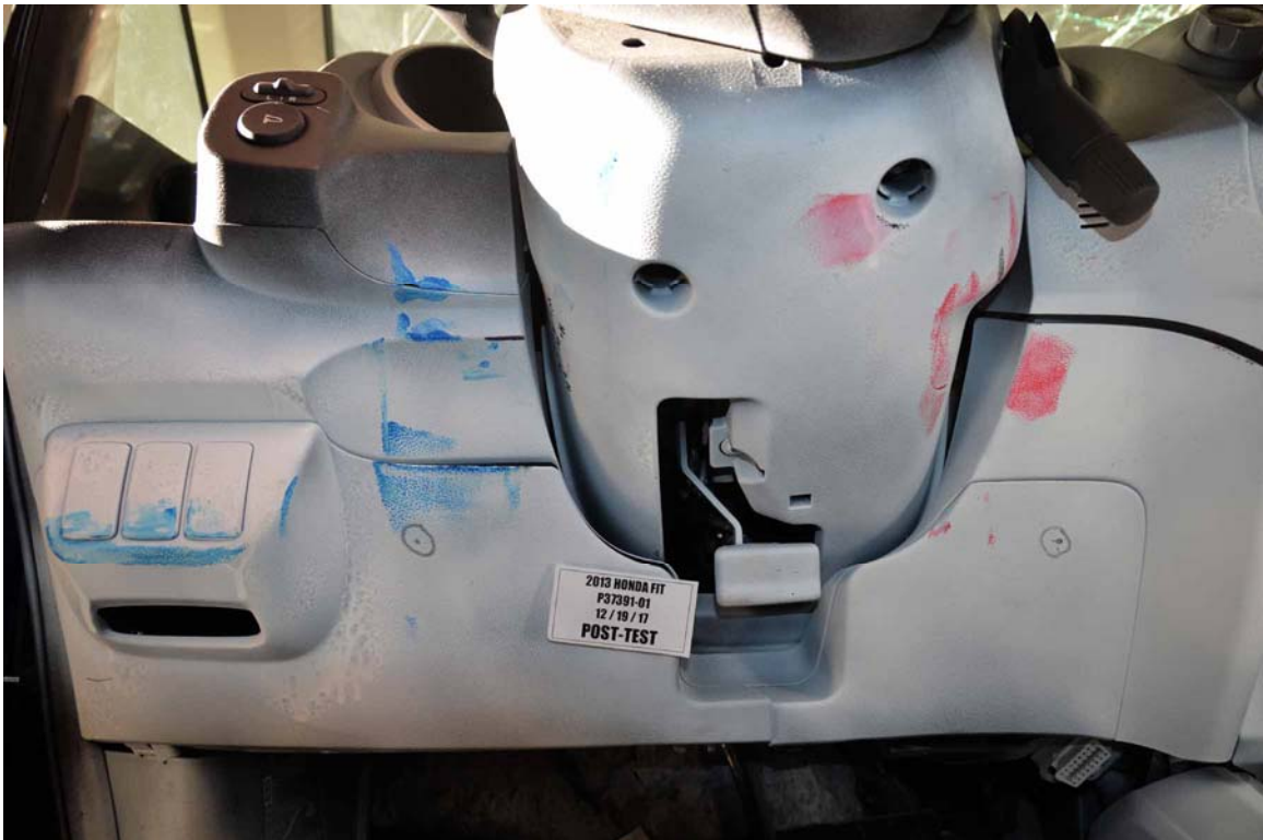
FIGURE 38. Post-Test Driver Dummy Contact with Knee Bolster
