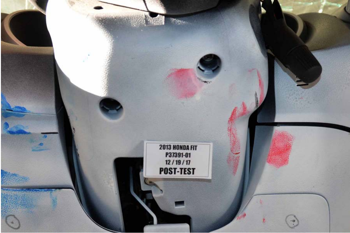
FIGURE 39. Post-Test Driver Dummy Contact with Steering Column
