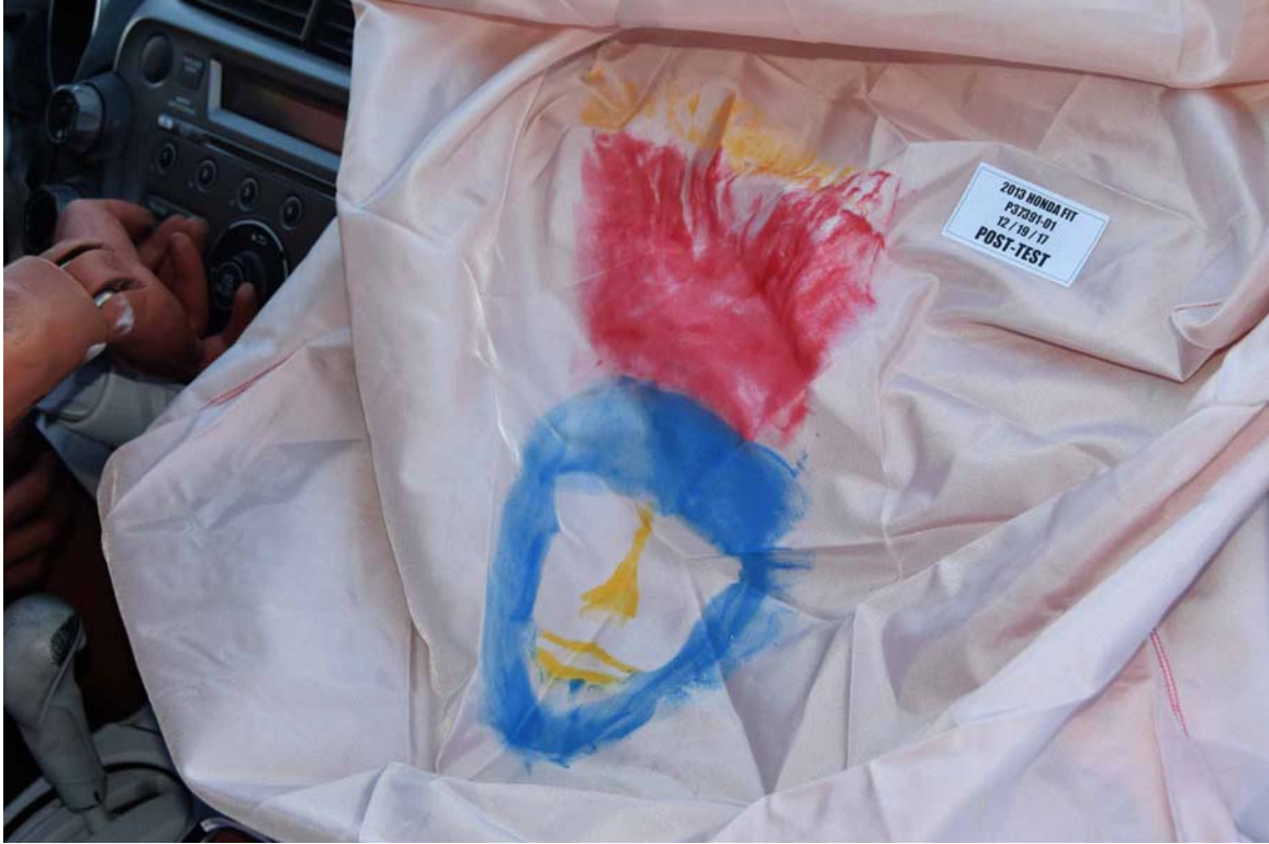
FIGURE 53. Post-Test Passenger Dummy Contact with Airbag
