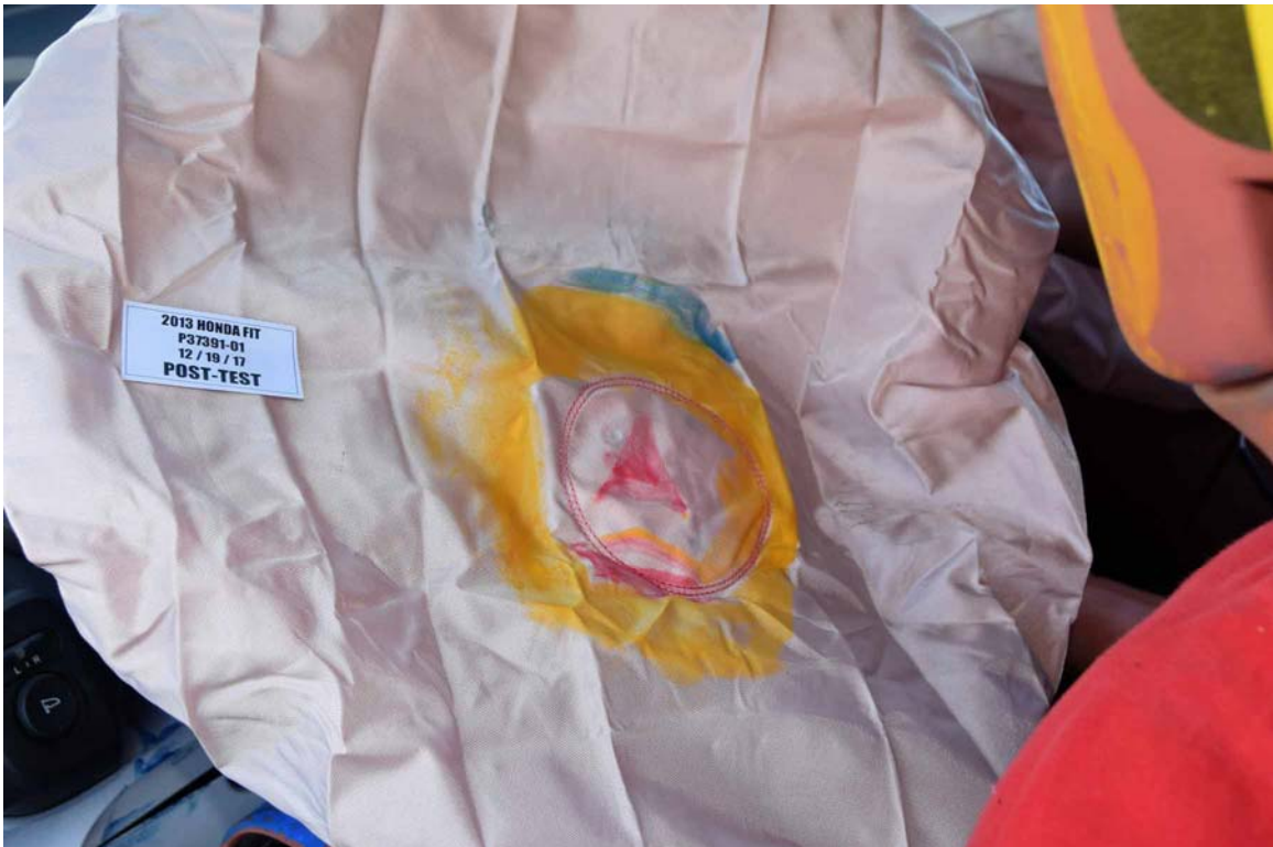
FIGURE 36. Post-Test Driver Dummy Contact with Airbag
