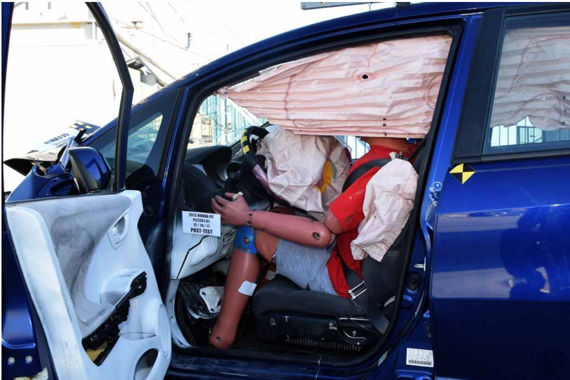
FIGURE 30. Post-Test Driver Dummy and Vehicle Interior
