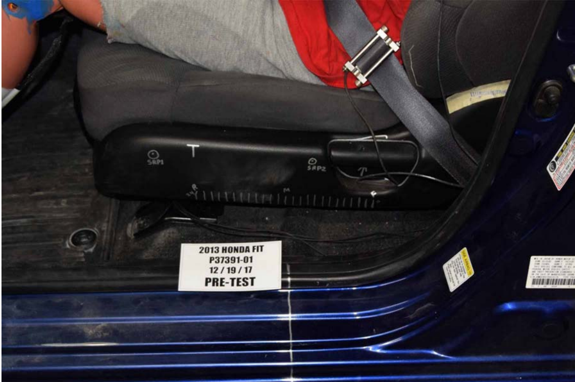
FIGURE 31. Pre-Test Driver's Seat Fore-Aft Markings
