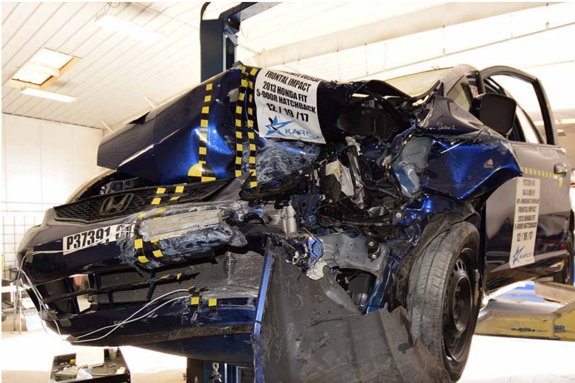
FIGURE 24. Post-Test Vehicle Impact Area
