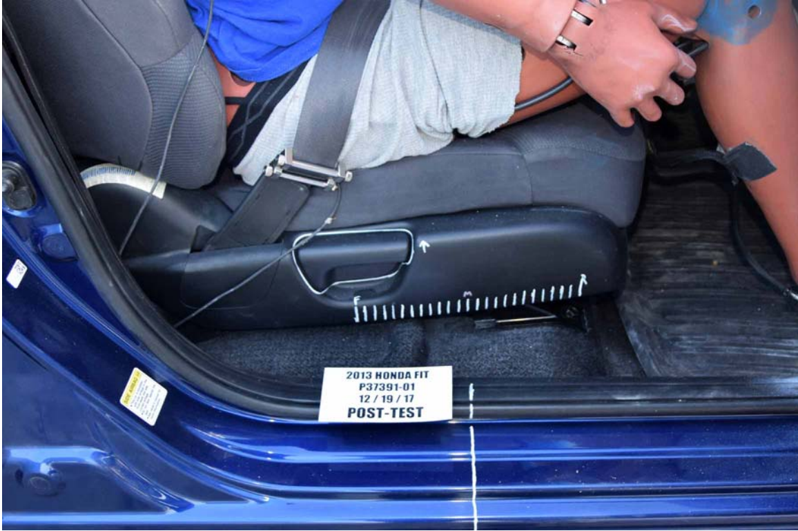
FIGURE 49. Post-Test Passenger's Seat Fore-Aft Markings
