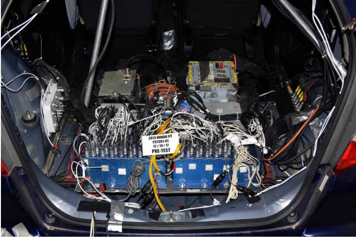
FIGURE 55. Pre-Test Equipment and Ballast
