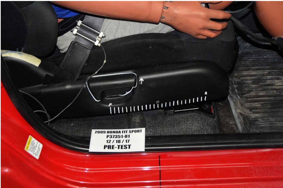
FIGURE 48. Pre-Test Passenger's Seat Fore-Aft Markings
