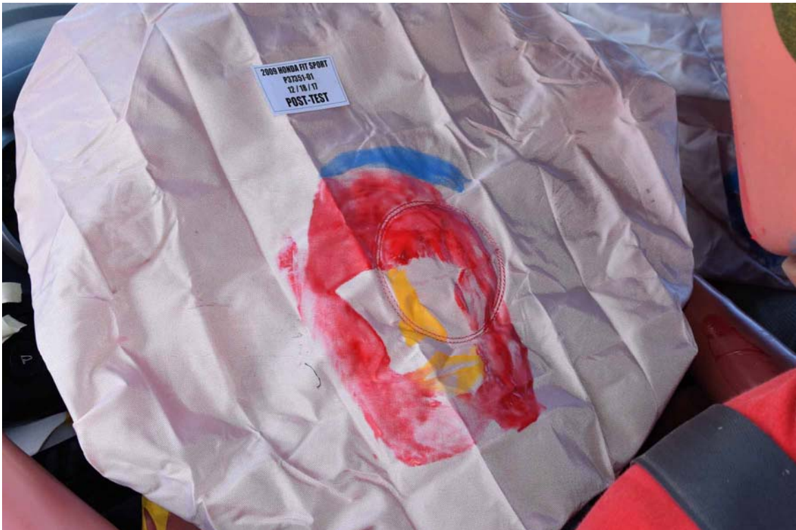
FIGURE 36. Post-Test Driver Dummy Contact with Frontal Airbag
