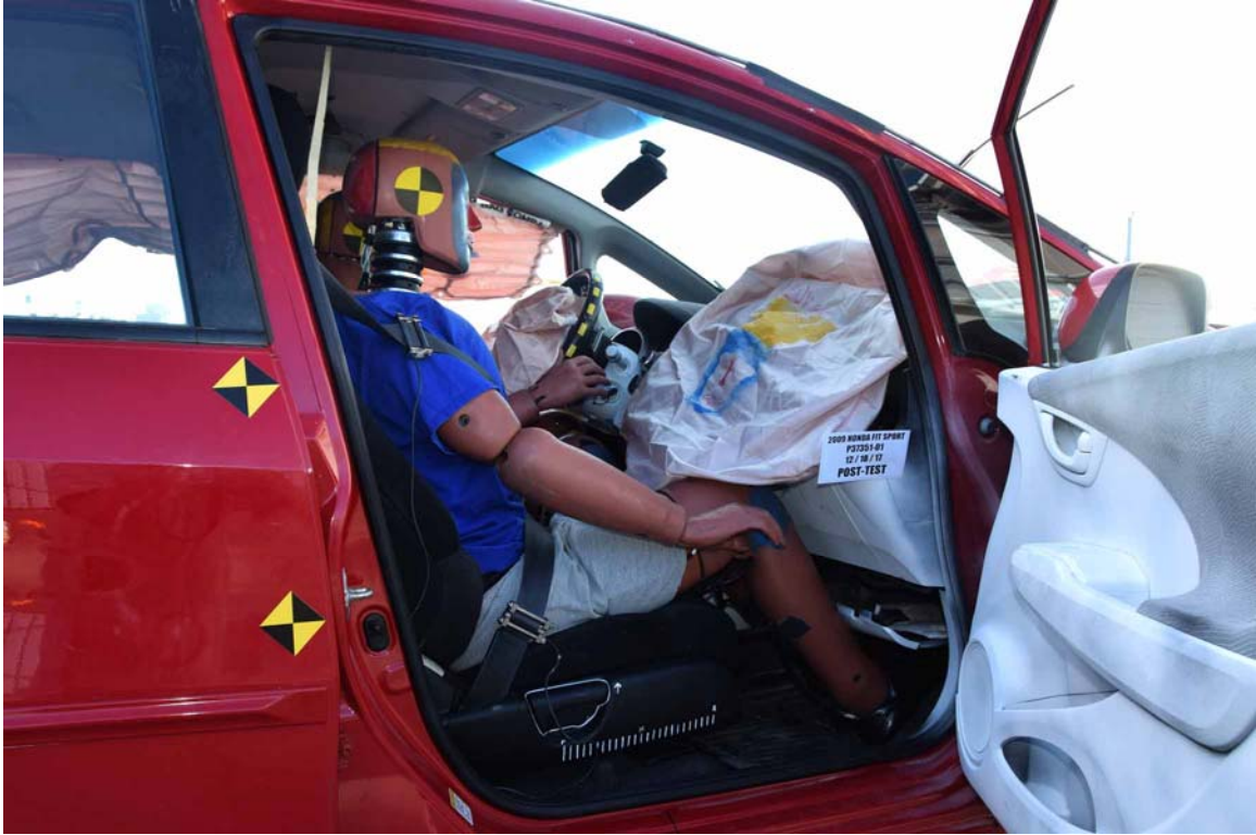
FIGURE 47. Post-Test Passenger Dummy and Vehicle Interior
