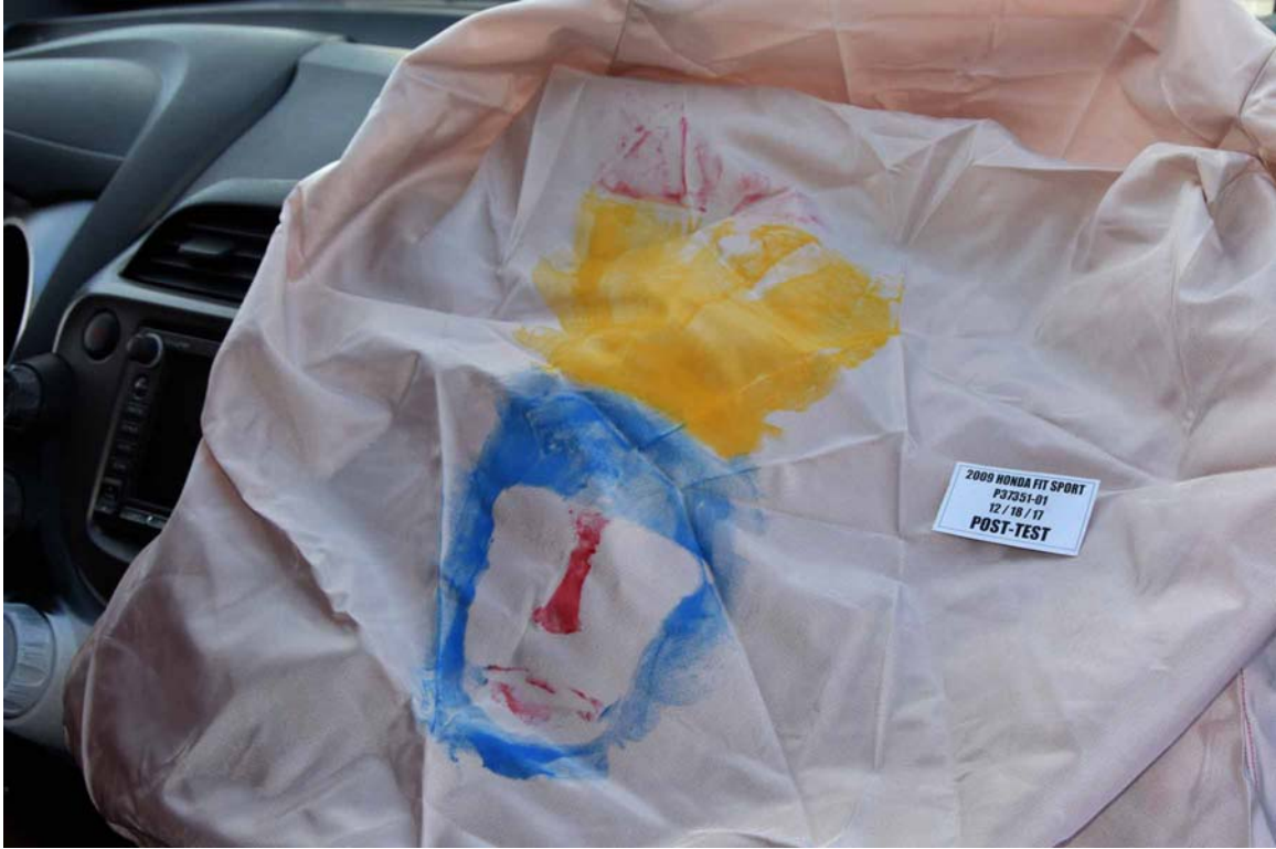
FIGURE 53. Post-Test Passenger Dummy Contact with Frontal Airbag
