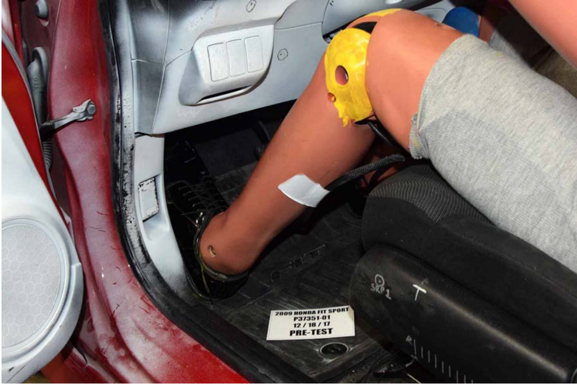
FIGURE 33. Pre-Test Driver Dummy Feet
