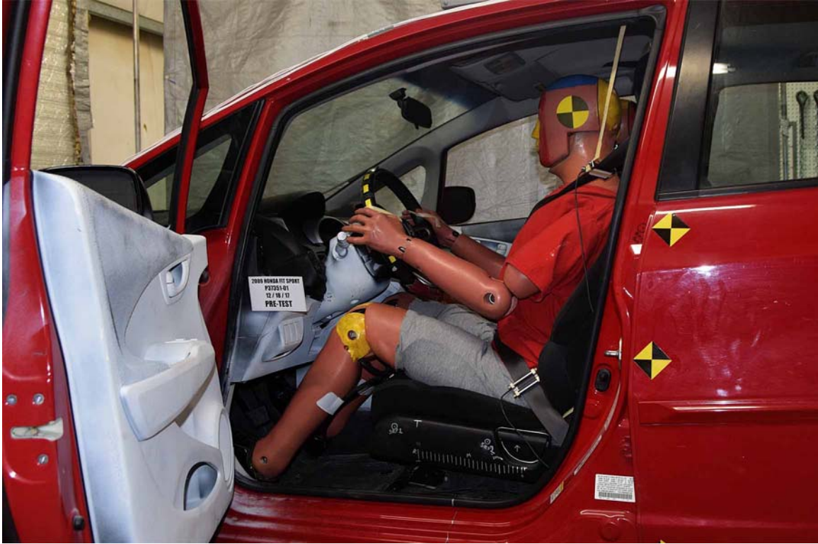
FIGURE 29. Pre-Test Driver Dummy and Vehicle Interior
