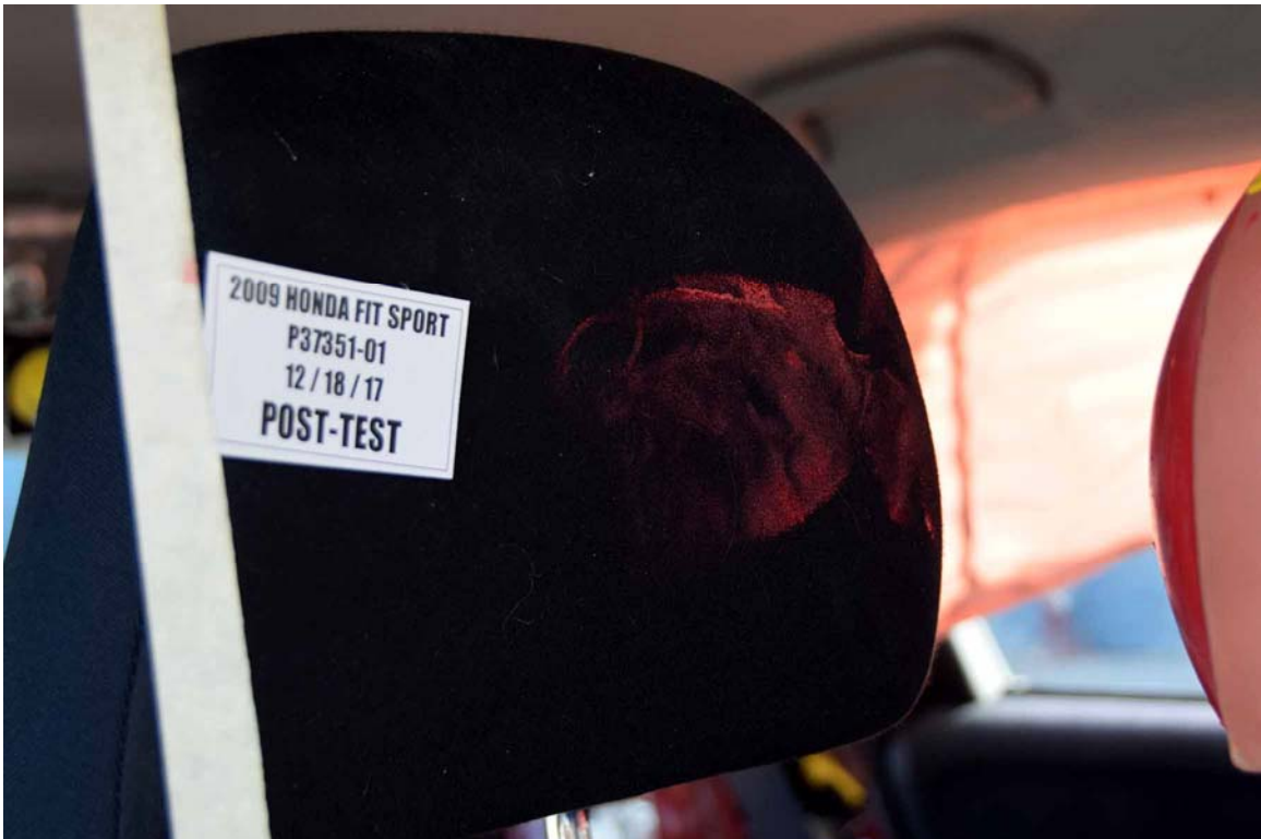
FIGURE 54. Post-Test Passenger Dummy Contact with Headrest
