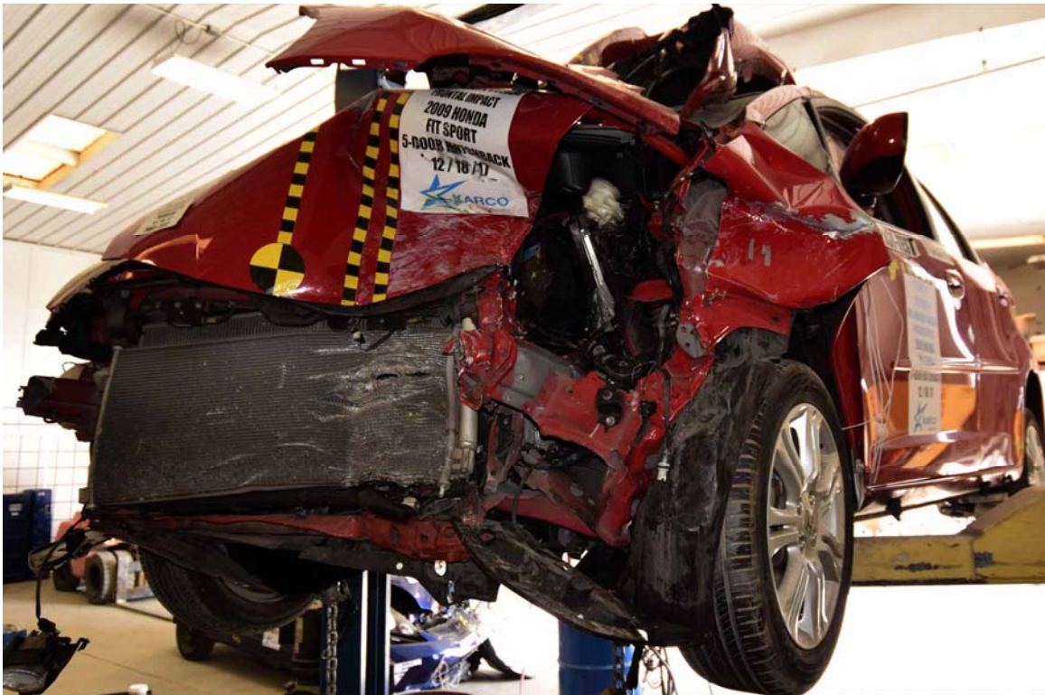
FIGURE 24. Post-Test Vehicle Impact Area
