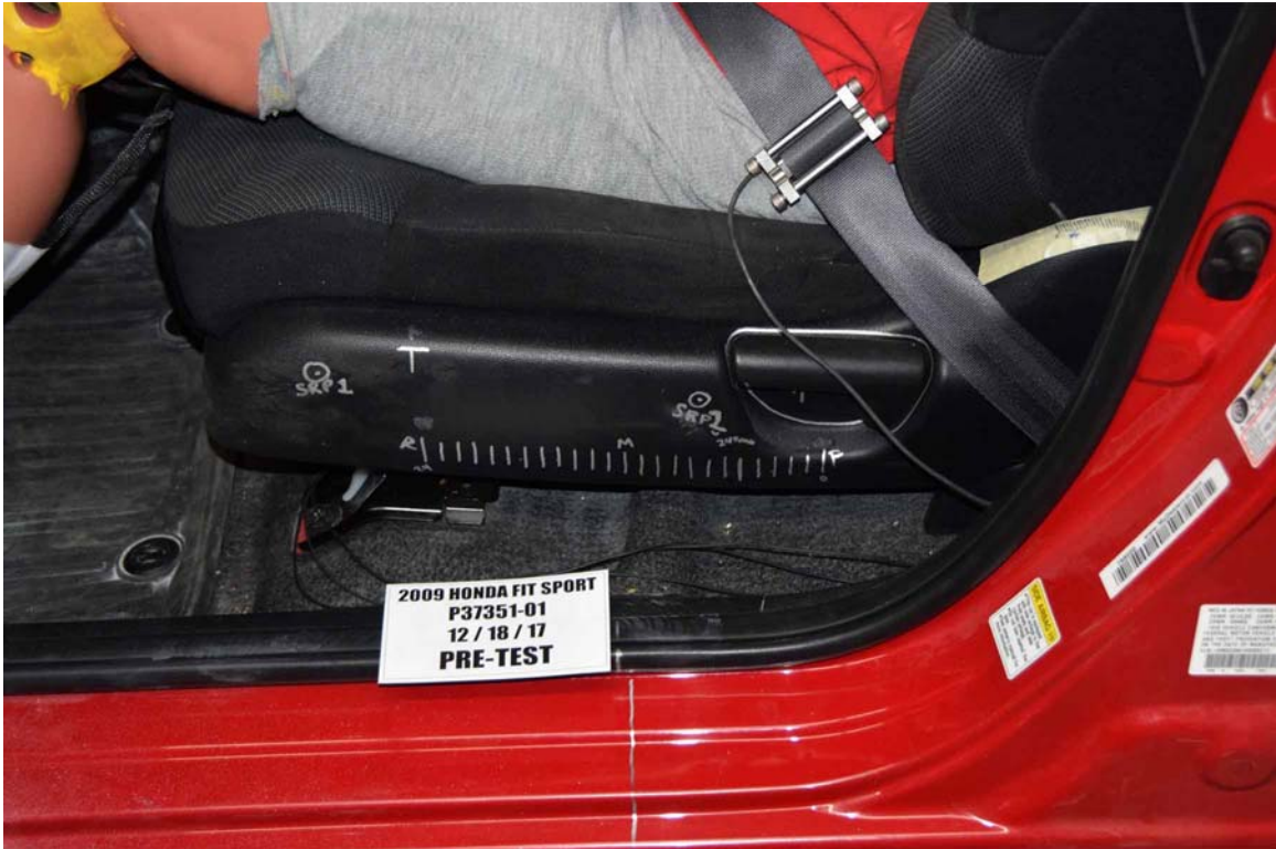
FIGURE 31. Pre-Test Driver's Seat Fore-Aft Markings
