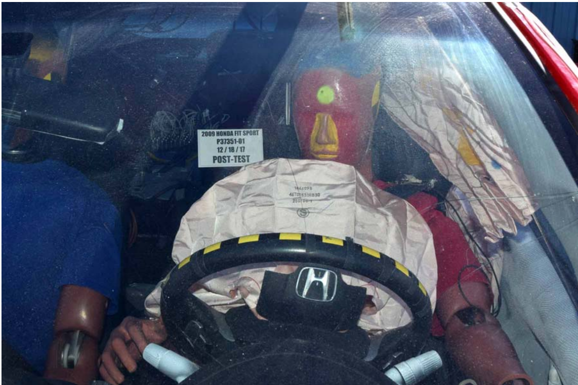
FIGURE 26. Post-Test Front View of Driver Dummy
