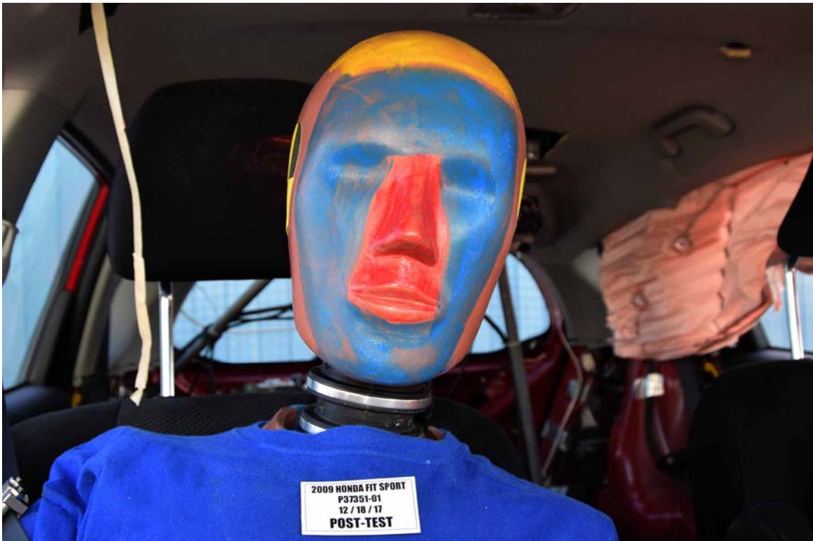
FIGURE 52. Post-Test Passenger Dummy Face
