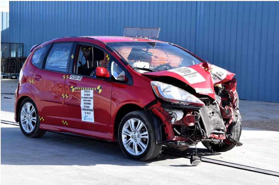
FIGURE 10. Post-Test Right Front ¾ View of Test Vehicle
