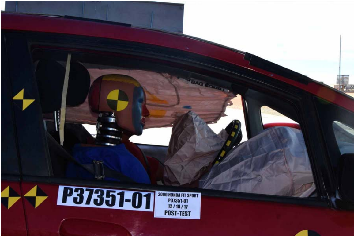
FIGURE 46. Post-Test Side View of Passenger Dummy
